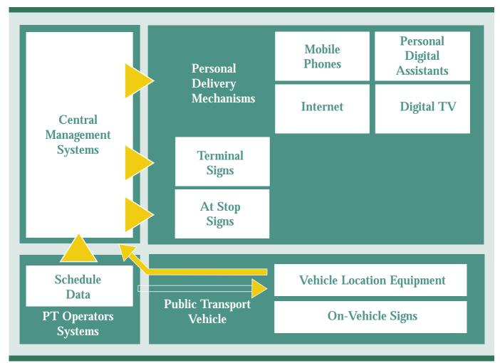
Schematic showing information delivery mechanisms
